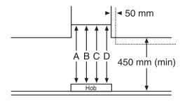
A: Built-in Electric Hob: 650mm minimum clearance
